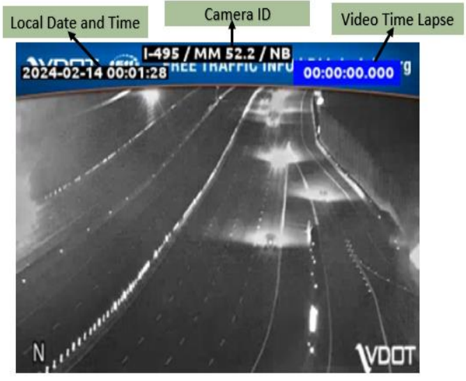
On-frame metadata overlays (date/time, camera ID, mile-marker, direction, elapsed time) parsed per clip for synchronization
