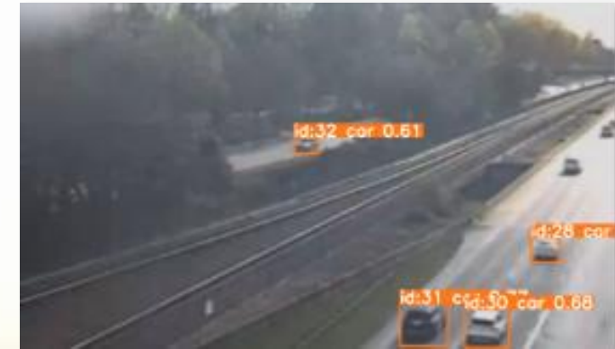
Evaluation of the Vehicle Detection Algorithm in Rainy Weather After Enhancement
