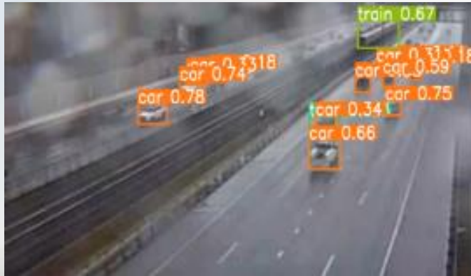
Evaluation of the Vehicle Detection Algorithm in Rainy Weather After Enhancement
