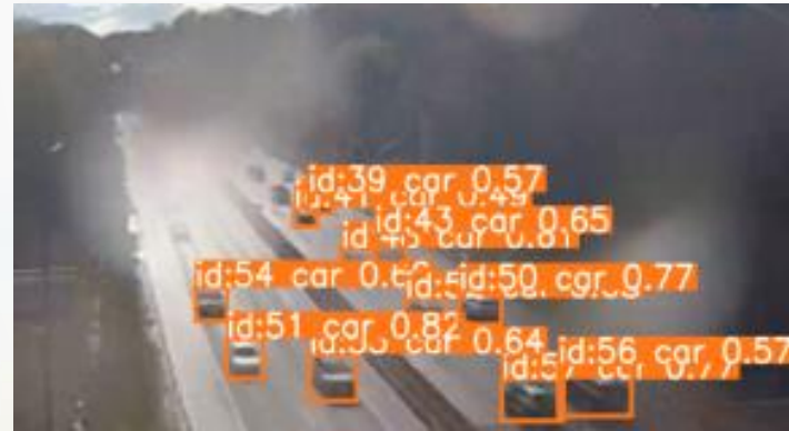
Evaluation of the Vehicle Detection Algorithm in Rainy Weather After Enhancement
